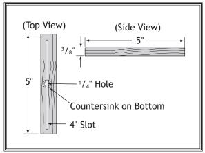
**Figure 65.** Patterns for featherboard miter bar.
